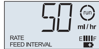
Figure 2-20 Pump is Running
