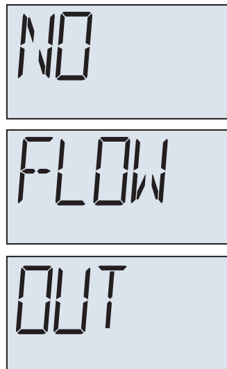
Figure 3-5 NO FLOW OUT Alarm
