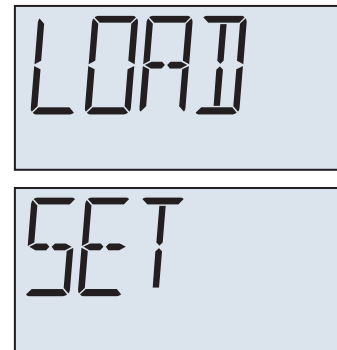
Figure 3-2 LOAD SET Alarm
