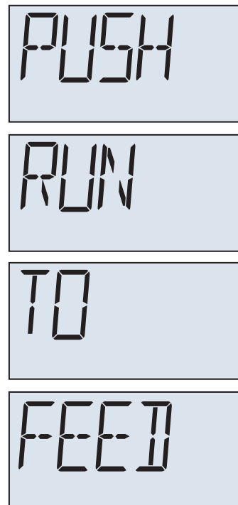
Figure 3-7 PUSH RUN TO FEED Alarm
