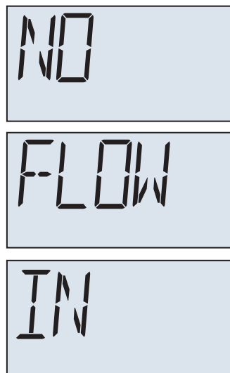
Figure 3-4 NO FLOW IN Alarm
