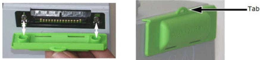
3. Ensure the tab points upward and press the cover firmly onto the IUI connector.
