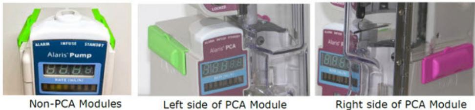
1. Inspect IUI connector covers for any damage. Do not use the cover if there is visible cracking, indentations, severe bending, or it is not fitting over the IUI connector.
