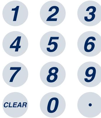
The [CLEAR] key will cause a highlighted numeric field to be cleared in preparation for data entry. It is also used to clear the displayed dashes (-- -- --) that occur when entering values beyond the pre-programmed hard limits. It WILL NOT clear the entire program.
