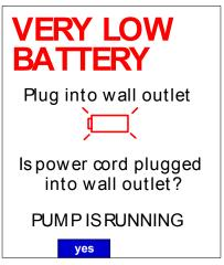
Figure 68. Very Low Battery Alarm.
