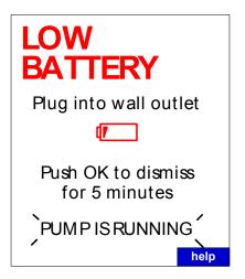
Figure 67. Low Battery Alarm.
