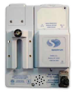
Figure 4. Back View - With Standard Battery (P/N 35724).
