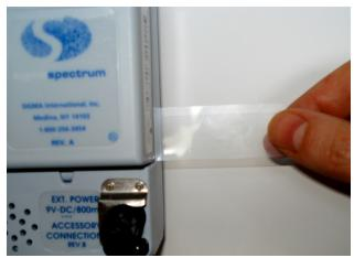
Figure 7. Battery Tab.
