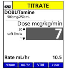
Figure 56. Titrate Screen with New Dose.
