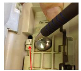
Cracked hinge on membrane frame
