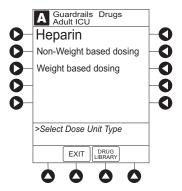
• If applicable, a weight-based or non weight-based option for delivery of this infusion could appear (as in illustrated example, which reflects use of Heparin).
