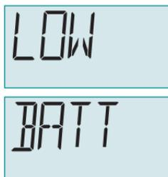
Figure 3-3 LOW BATT Alarm
