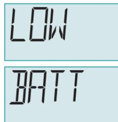
Figure 3-3 Alarme LOW BATT (pile faible)
